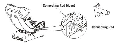
▶ There are brackets located at top and bottom of the armrest to connect it to the main body. Attach the armrest to the top and bottom brackets. Secure with 4 screws on the bottom bracket, and 2 screws on the top bracket.
