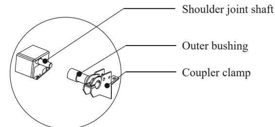
▶ Remove the screw off the coupler clamp, latch upwards to unlock it, fit the footrest joint shaft to the coupler hook and latch downwards to lock it, tighten the screw. (Check below illustration for reference)
