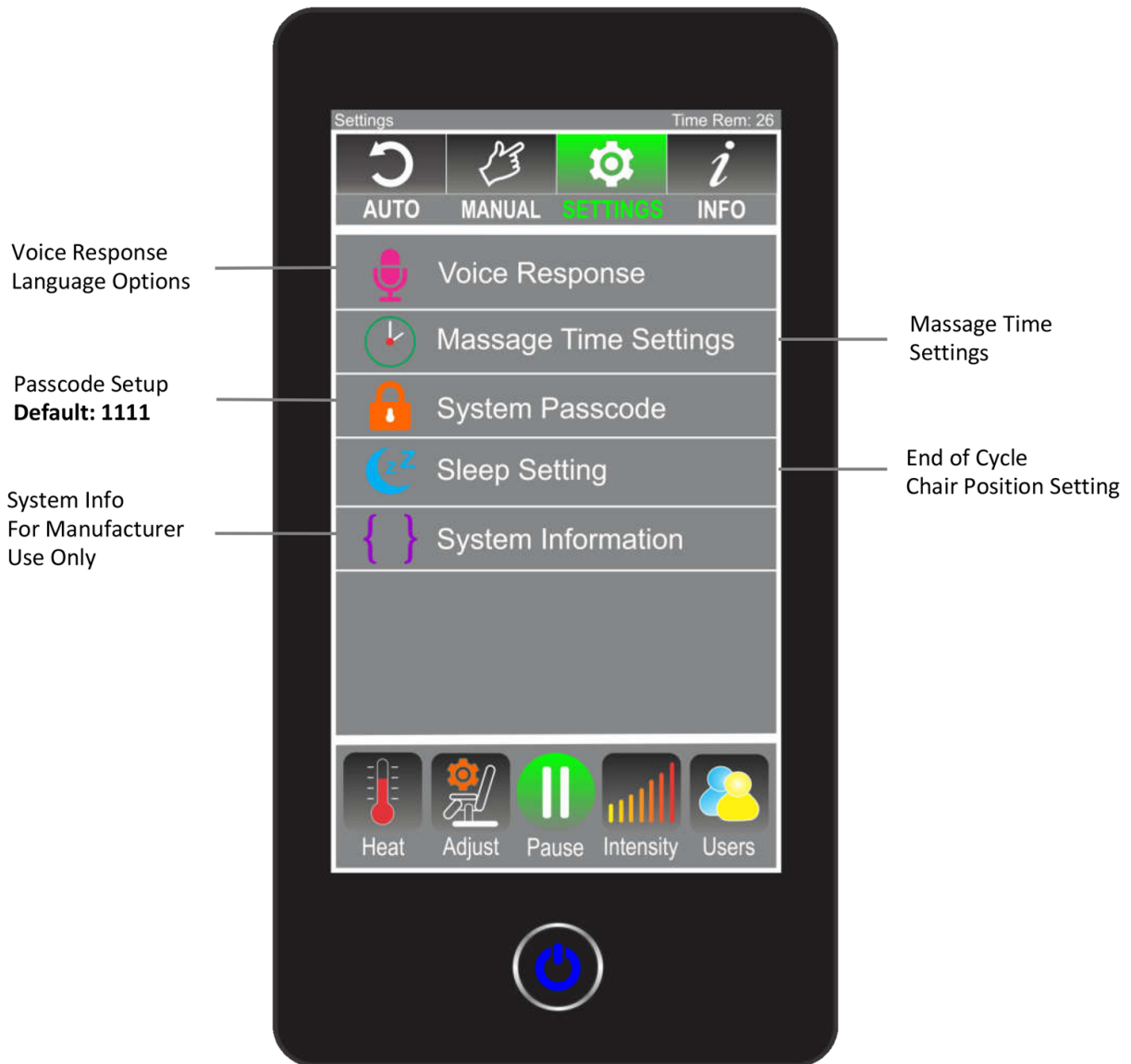
Fig.11: System Setting Description
