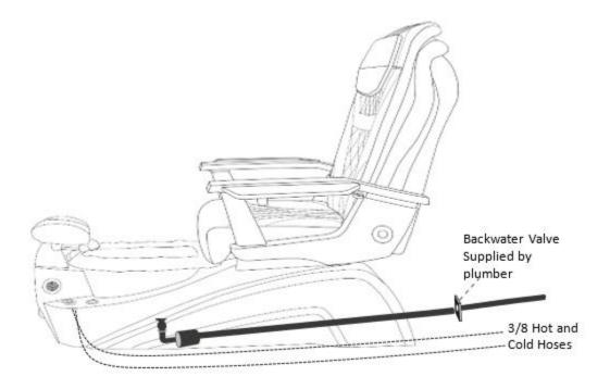
Typical Gravity Sink (Direct Drain) Installation
