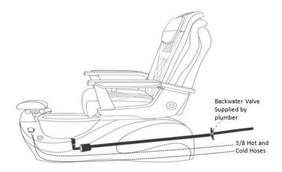
Typical Gravity Sink (Direct Drain) Installation
